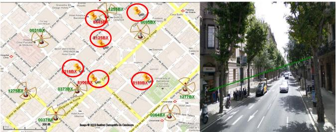
Background: intra-frequency deployment with 4 Macro and 6 Micro cells, improve the street coverage and offload capacity
